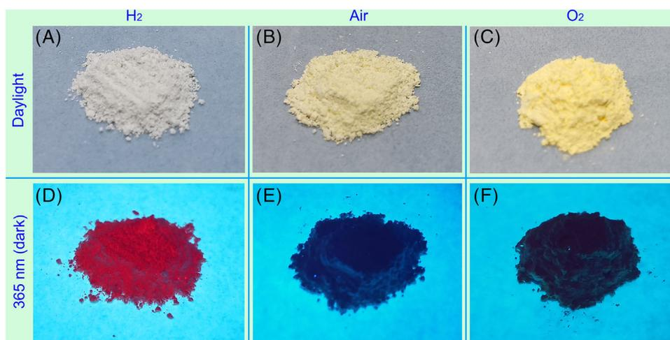
FIGURE 8 Macroscopic appearance of the different Pr6 pigments, (A, B, and C) in daylight and (D, E, and F) activated by a 365-nm UV lamp in dark; (A and D) H<sub>2</sub>-based, (B and E) air-based, (C and F) O<sub>2</sub>-based.
